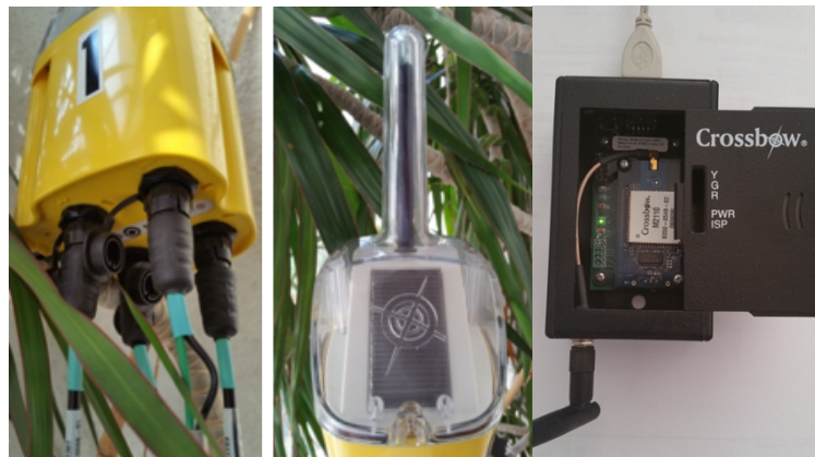
Figure. 3.3. The wireless node and the base-radio.
