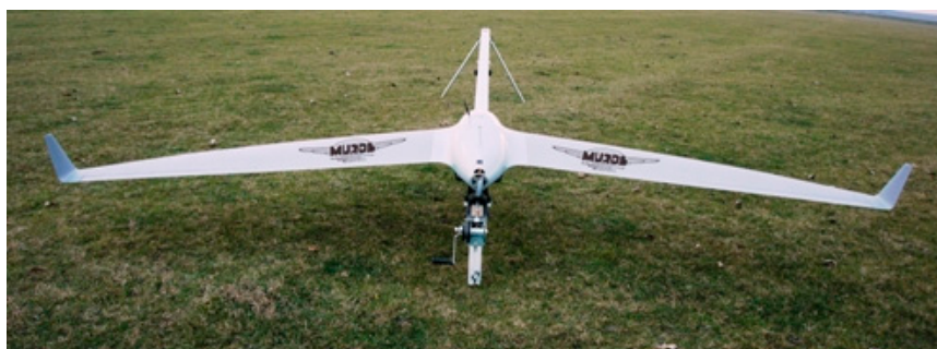
Figure 2. UAV MUROS on launcher.
