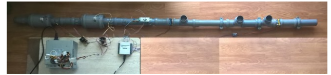
Fig. 6. Experimental installation (with real sensors and actuators). Fails are provoked by removing pipe caps – right part.
